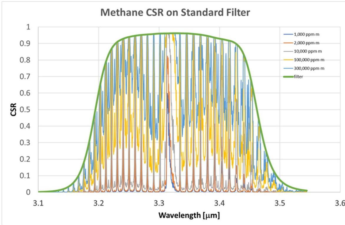
Figure 2 compounds specific response spectrum and the camera SF, for a wide range of CL values.
