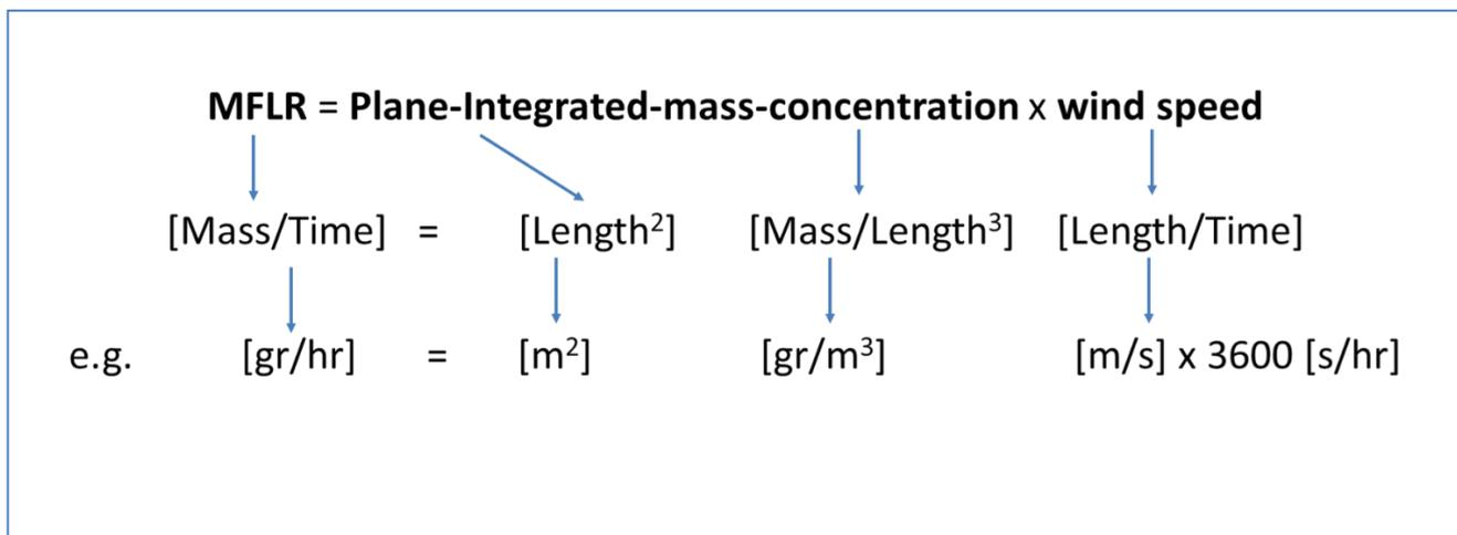
Figure 1. The retrieved components from a series of OGI images for calculating MFLR
