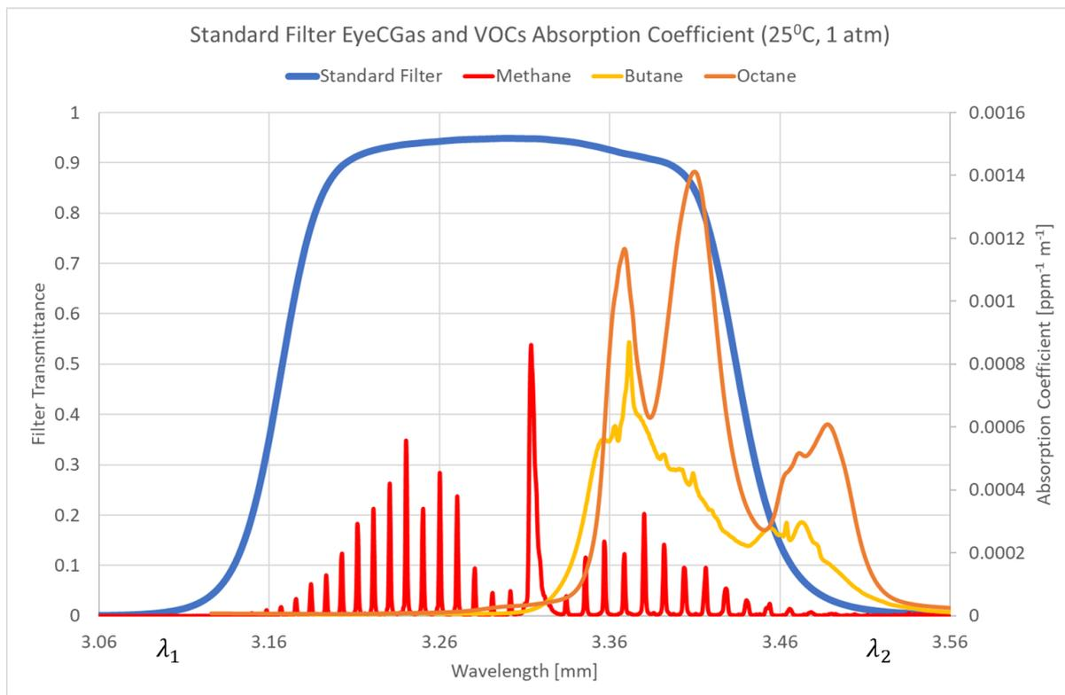
Figure 1 Examples of absorption coefficient curves for 3 VOCs and EyeCGas2.0 standard filter transmission
