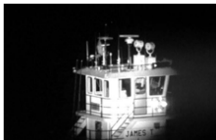
A near-IR laser illuminator uses a covert, continuous-wave, adjustable laser to produce natural-contrast video in which text can be read, people identified, behavior recognized, and critical scene details observed at more than 4,000 meters away at night and more than 15,000 meters during the day.
